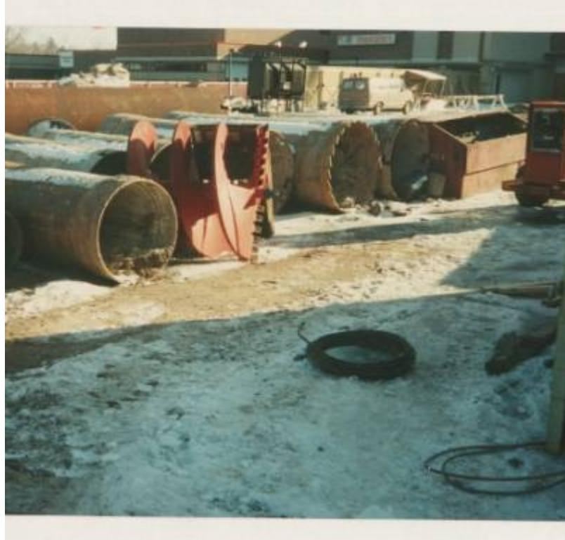
Fig. 14. Drill bits and shafts used to install drilled piers.
