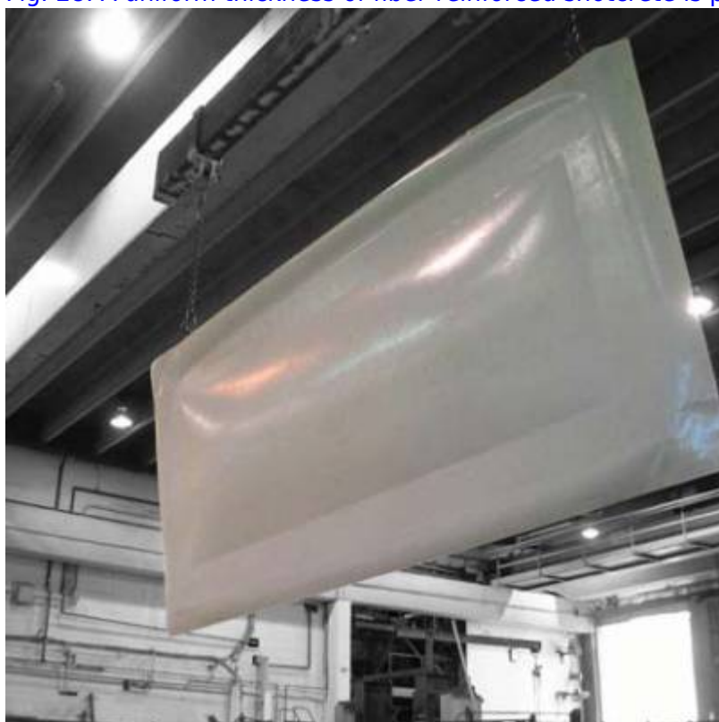
Fig. 29. Completed prototype plastic-coated mold.
