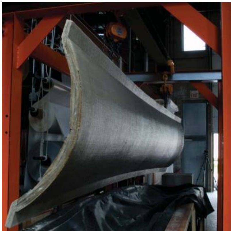
Fig. 35. Removing 3 cm (1.2 in) vault from formwork.
