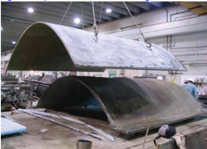
Fig. 23. Step 2- Uniform layer of GFRC is applied.
