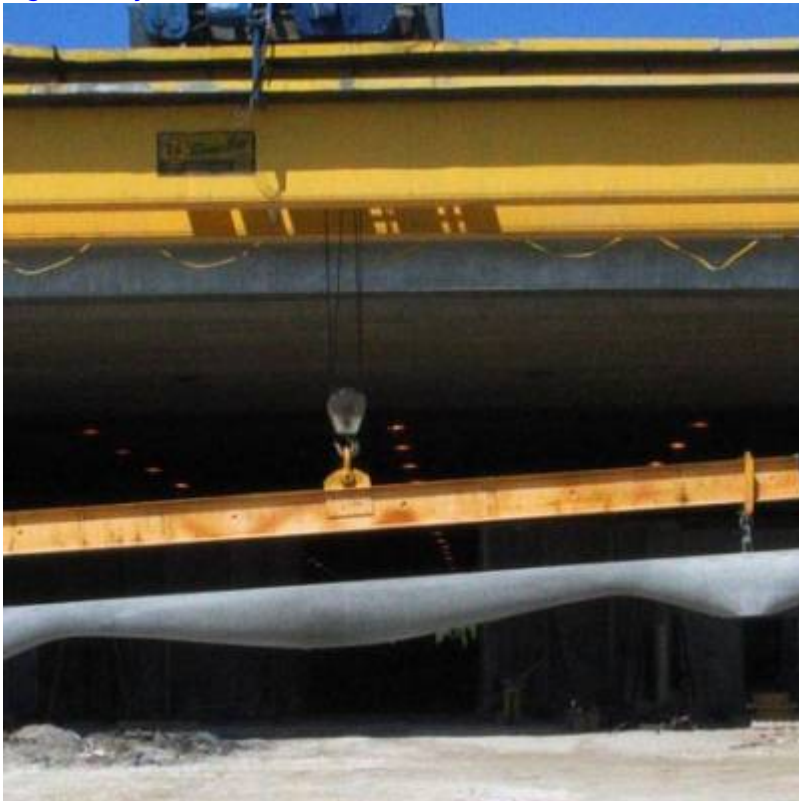
Fig. 12. Completed full scale variable section concrete beam.
