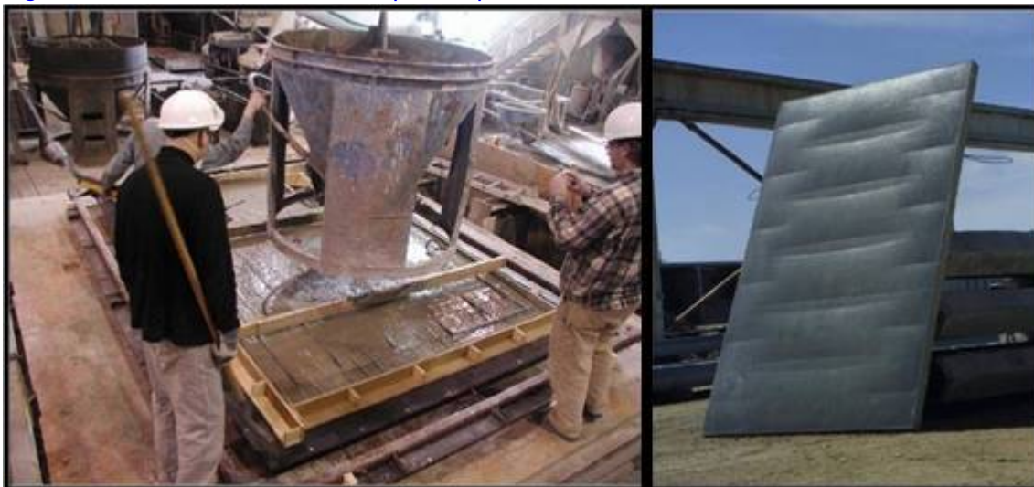
Fig. 2. Full-scale formwork and completed concrete panel.
